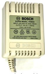
TF008-B Power supply plug pack is used with Solution 2000 / 3000 / 4000 / 6000 control panels. The plug pack includes built-in thermal fuses that blow during overload or fault conditions to eliminate a possible fire threat due to excessive heat buildup inside the casing.
