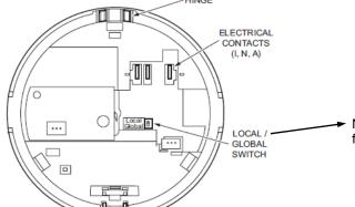
NOTE - Local/Global Switch - defines the relay trigger function on the optional 755RB relay base only.
