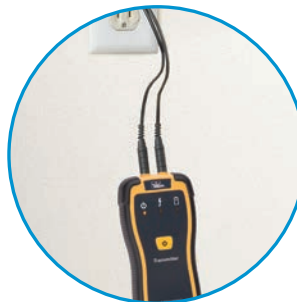
Traces on de-energised circuits
