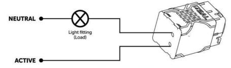
ALLOWABLE LOADS: INCANDESCENT & HALOGEN - 600W; LED - 400VA; FAN - 120VA
