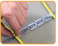
3259 Galvanised Fixing Profile A 25m roll of galvanised steel fixing profile. Can be mechanically fixed to timber or concrete substrates. Allow 1m of fixing strip per 6m of heating cable.
