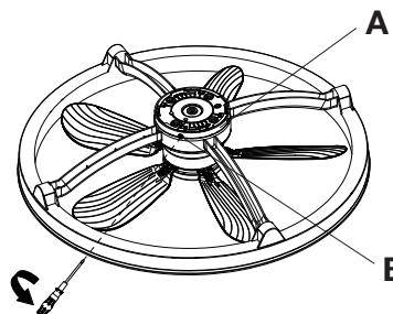
3. Rotate the wall mounting plate "C" from light body "A" counter-clockwise to unlock the safety lock "D"
