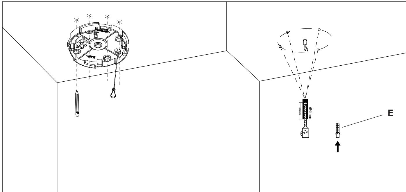
5. Use screws "F" provided to secure the wall mounting plate "C" onto a flat ceiling surface.
