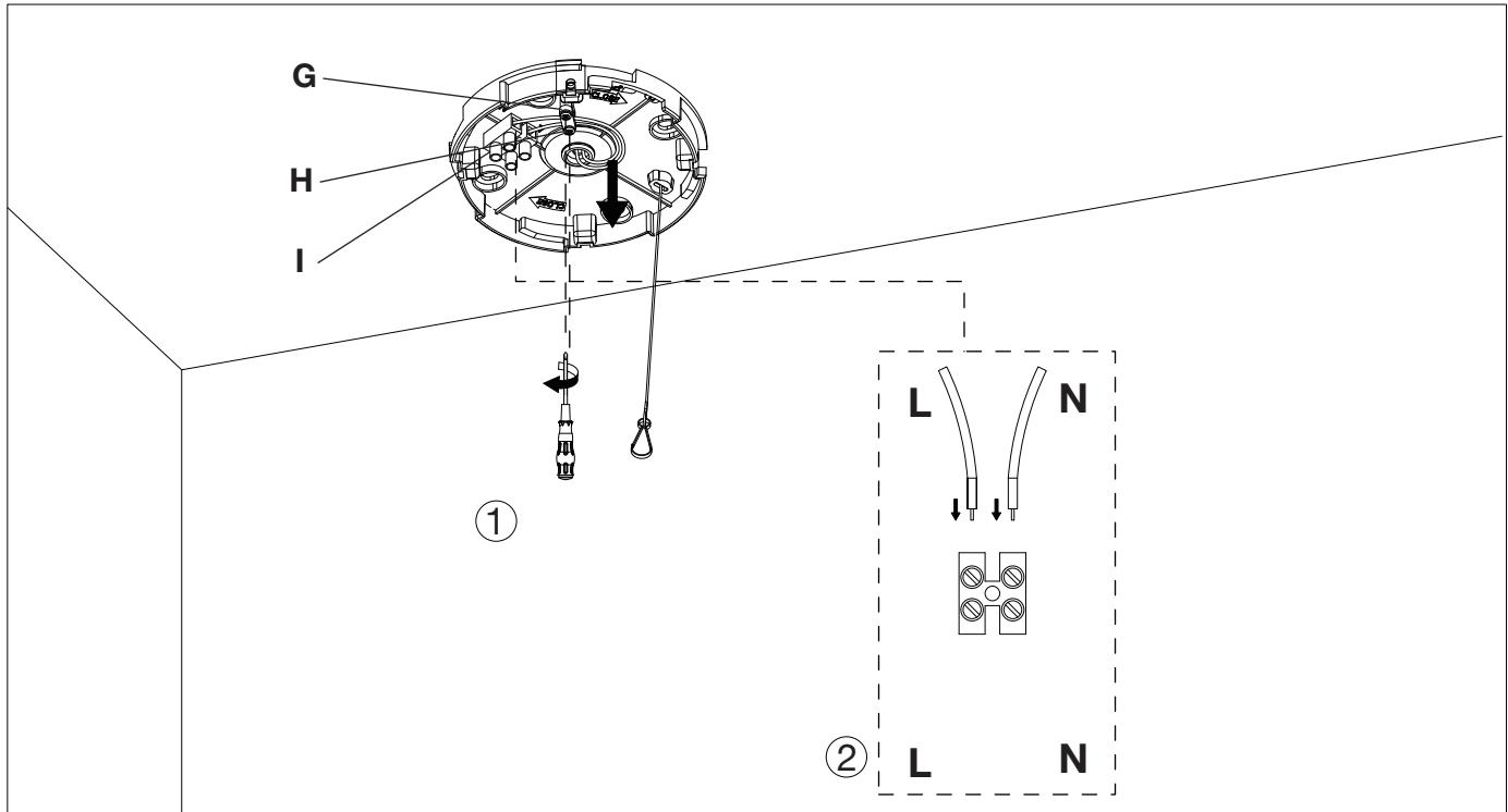
7. Connect the drive live "L" and neutral "N" wires to the terminal "I". Secure the terminal block "G" to part "C" using 2 screws "H".
