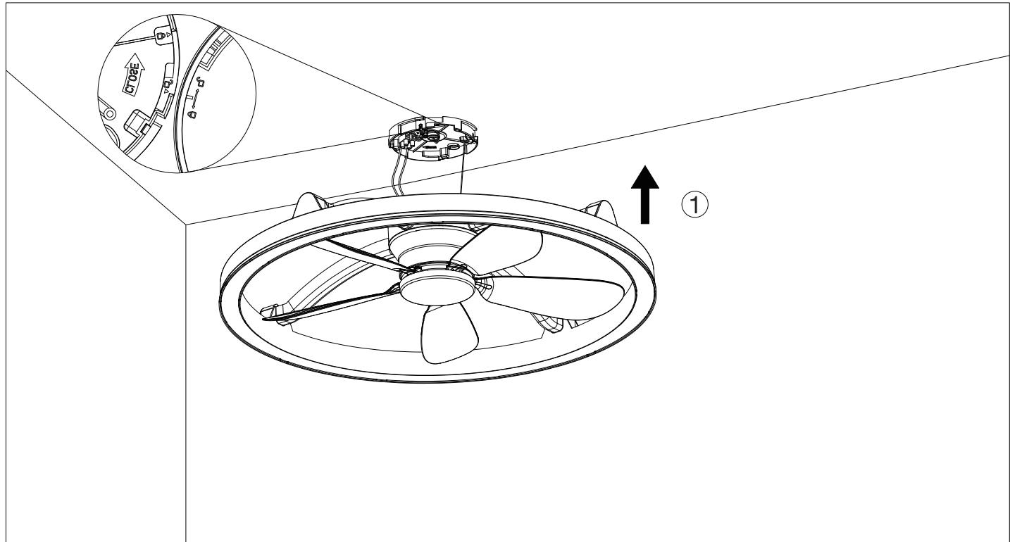
9. Use a screwdriver to tighten the 4 screws "B" on part "A" by turning them clockwise.
